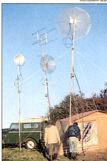
The South Birmingham Radio Society (G8OHM/P, G1OHM/P, G3OHM/P and G4JNT/P) sported this antenna farm for the 1.3, 3.4, 2.3 and 5.7GHz bands during the October 1990 '432MHz and up' Contest.
